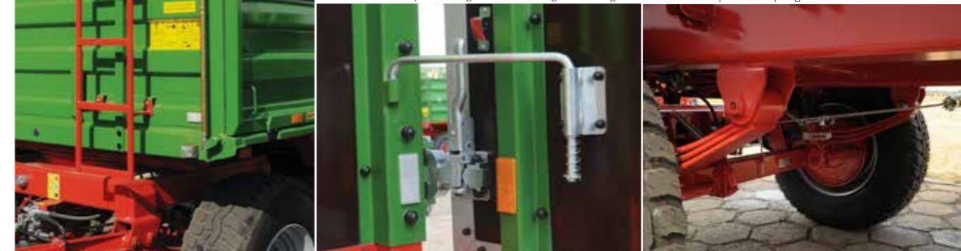
Sidewall blockade protects against self-closing and damage
